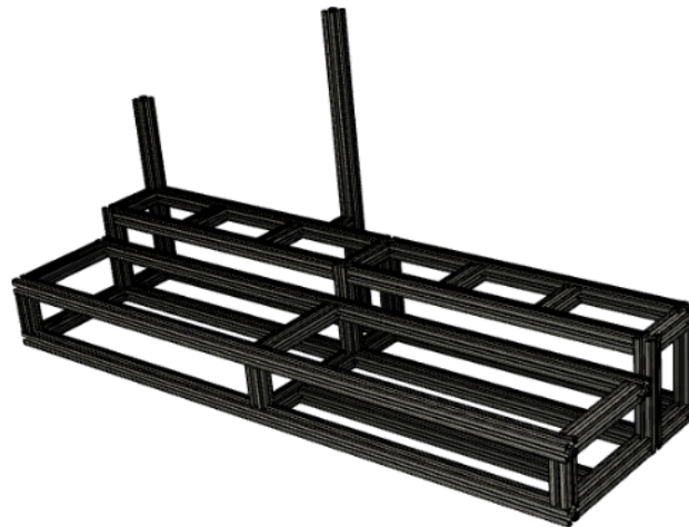
Figure 4: Main frame for automated cleaning machine prototype
