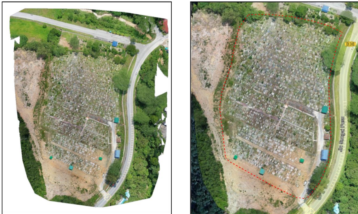
a) Orthophoto output from Pix4D processing result b) Orthophoto overlay with open-source map
