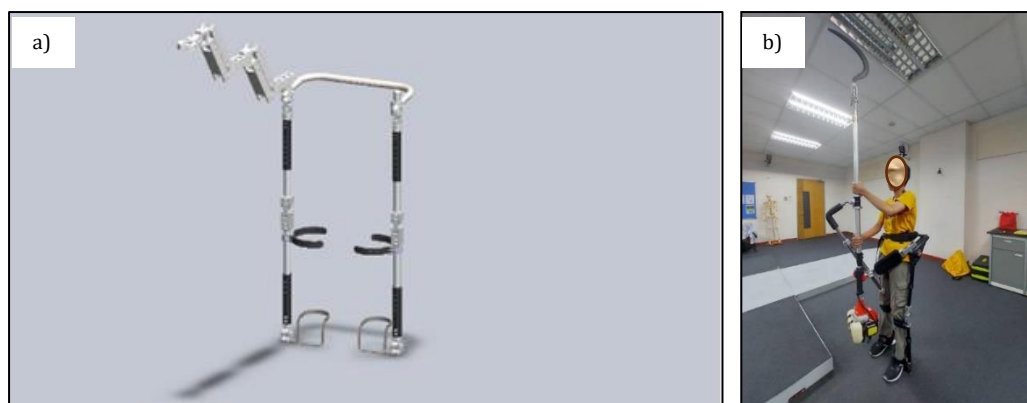
Figure 3. a) 3D Rendering of EXOROBO b) Subject Performing Simulated Walk-and-Carry Task
