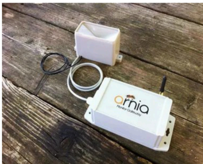
Figure 7. Arnia remote hive monitoring system [10].
