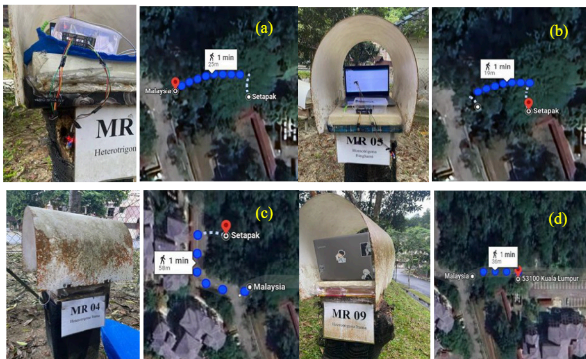
Figure 25. Hive located at (a) 19 meters, (b) 25 meters, (c) 36 meters, and (d) 58 meters elevated from the LoRa gateway node.
