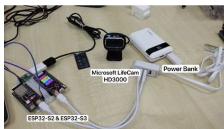
Figure 1: System setup using ESP32-S2 and ESP32-S3
