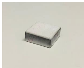
Figure 2: Specimen size: 15mm x 15mm x 6mm.
