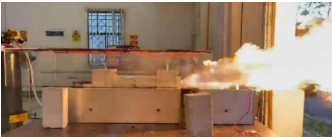
Figure 10: Four port with oxidizer pressure of 100 kPa
