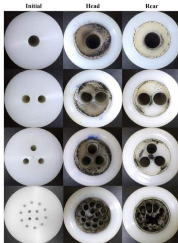
Figure 3: Final ports of the head and back end of the cross-sectional configuration of the HDPE solid fuel grain both before and after the test of hot firing for 1 port, 2 ports, 3 ports and 14 ports [16]
