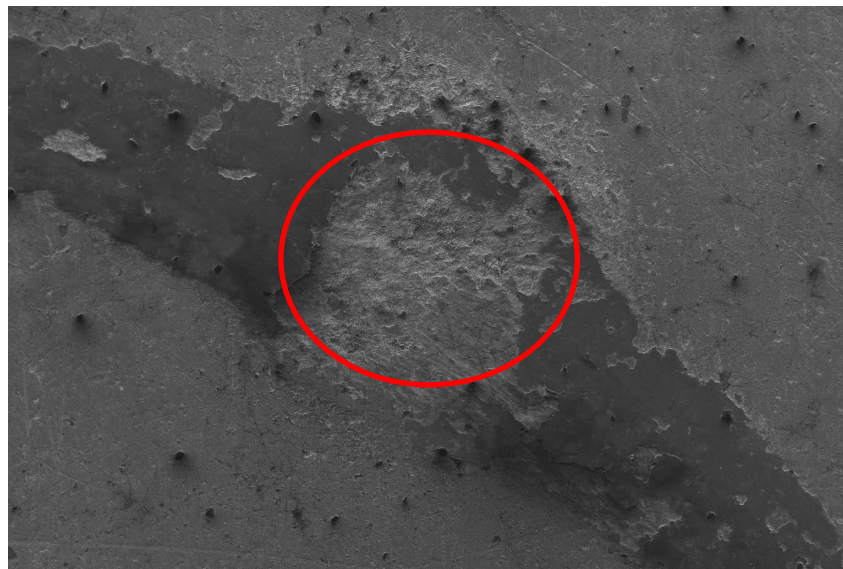
Fig. 8. Images of the trapped debris in the crater
