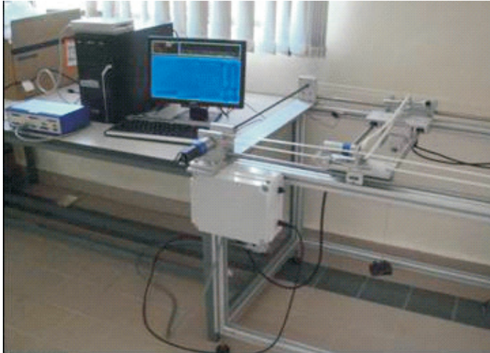
Figure 2. Lab-scale gantry crane prototype.
