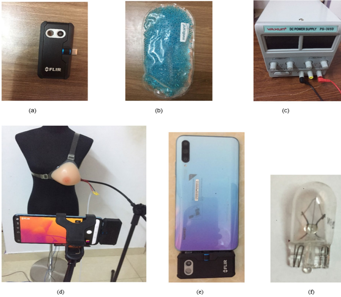
Fig. 6 Materials used: a FLIR One Pro thermal camera, b cooling gel, c DC power supply, d 1 m distance between breast and thermal camera, e FLIR One Pro connected in mobile phone and f lamp (12V5W) with 1 cm diameter
