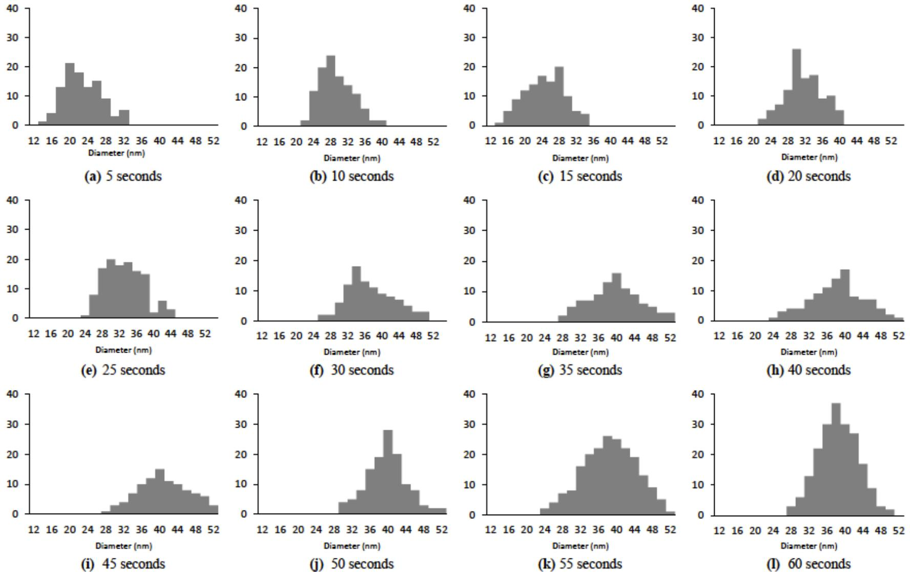
**Fig. 3:** CNT diameter distribution at 5 seconds increment. (a)-(f) marks the transient stage where average diameter increases while (g)-(l) shows a steady distribution of CNT diameter when exposed into flame under the same flame condition
