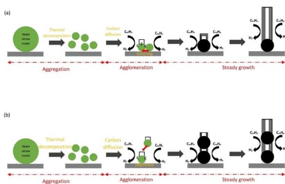
**Fig. 6:** Formation of catalyst nanoparticle and growth of CNT based on the aggregation-agglomeration-sintering process. (a) Particle sintering that leads to increase in particle size and carbon diffusion rate to form large nanotube diameter. (b) Particle deposited on top of another to form a long strand of CNT with multiple particles in between.
