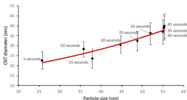
**Fig. 8:** Correlation between carbon nanotube diameter and catalyst particle size at various sampling times. The instantaneous reactions show that the formation of both particles reached a uniform size after 36 second sampling.
