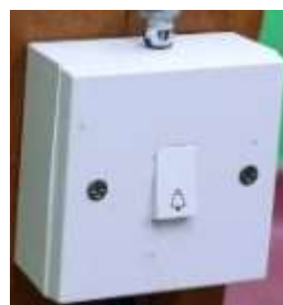
Figure 4. The front desk switch and the kill switch located on the top.
