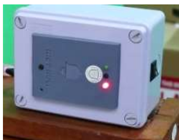
Figure 3. Circuit box and the touch switch represented by the bell icon.
