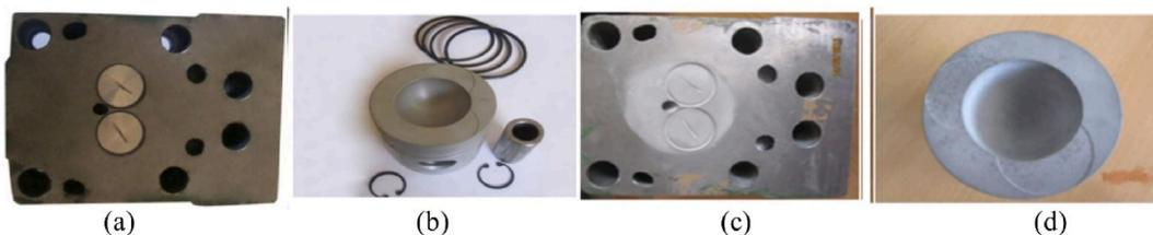
**Fig. 3.** a–d. Diesel engine hardware components include (a) uncoated cylinder head and valves, (b) uncoated piston, (c) coated cylinder head and valves, and (d) coated piston.
