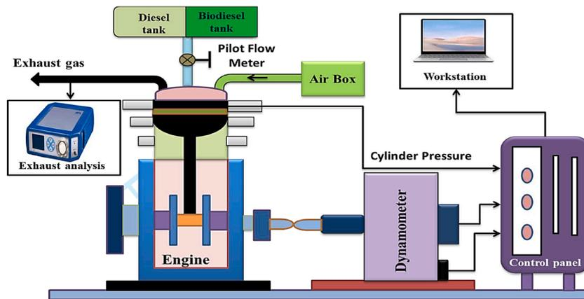
Fig. 4. The engine test setup.
