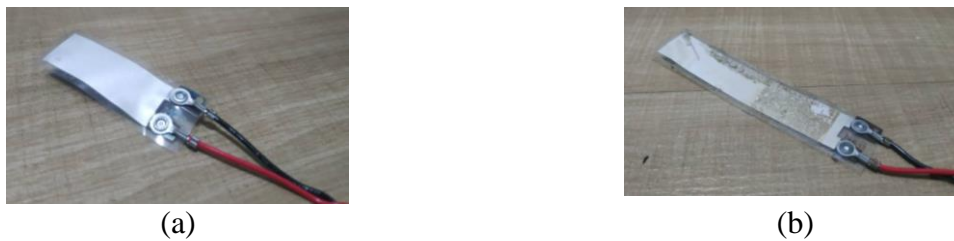
Figure 2: PVDF thin films used in the experiment. (a) 16 mm x 41 mm x 40\mu\text{m} and (b) 16 mm x 73 mm x 40\mu\text{m}
