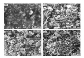
**Fig. 1** FE-SEM micrographs of (a) pristine PAI and NCs containing (b) 5 wt%, (c) 10 wt%, and (d) 15 wt% modified MWCNTs.
