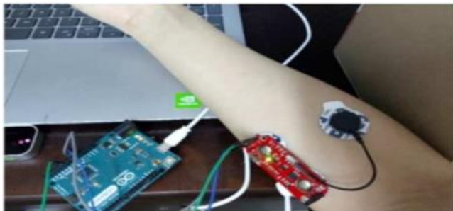
Fig. 3. The MyoWare muscle sensors on the arm. Source: Adapted from [5]
