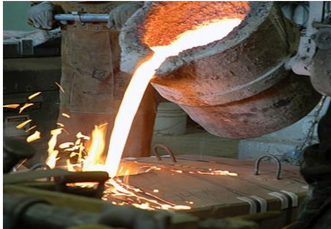
Fig. 6, Casting- pouring molten metal into mould is risky to human being and environment.
