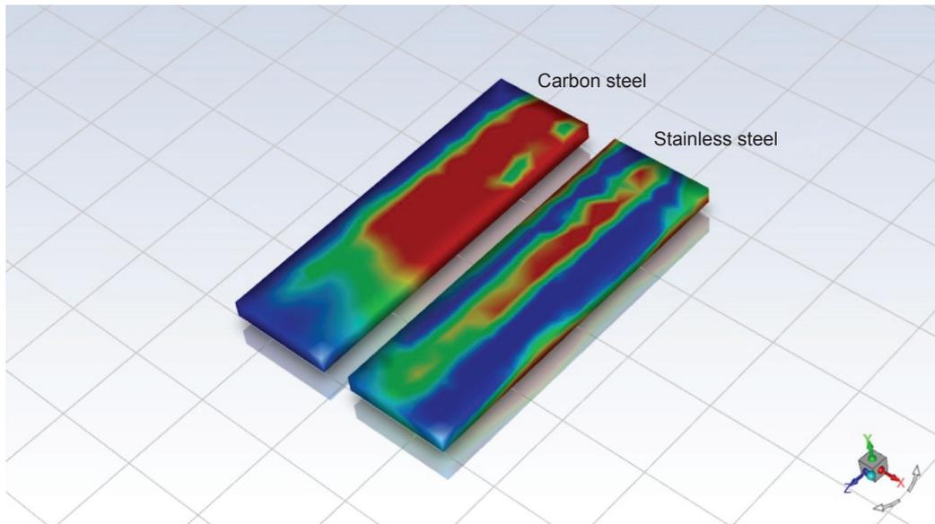
Figure 5. Corroded surfaces of carbon steel and stainless steel after biodiesel exposure.
