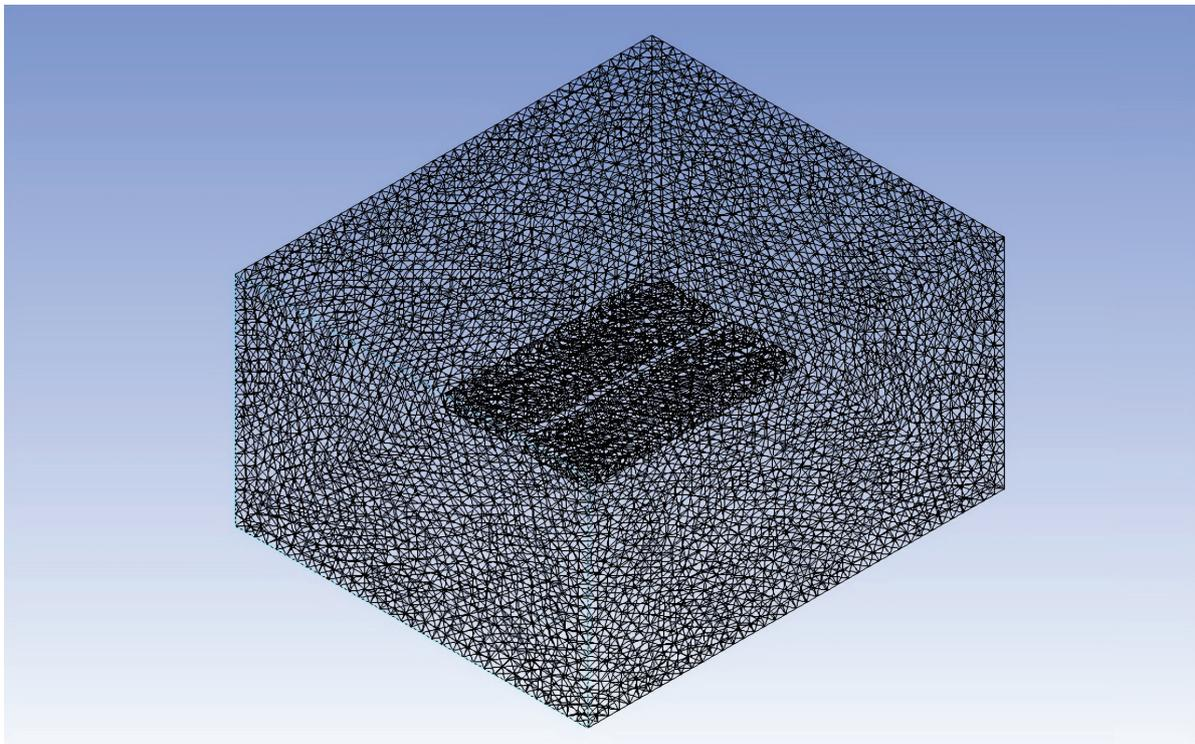
Figure 2. Meshed geometry of corrosion analysis.
