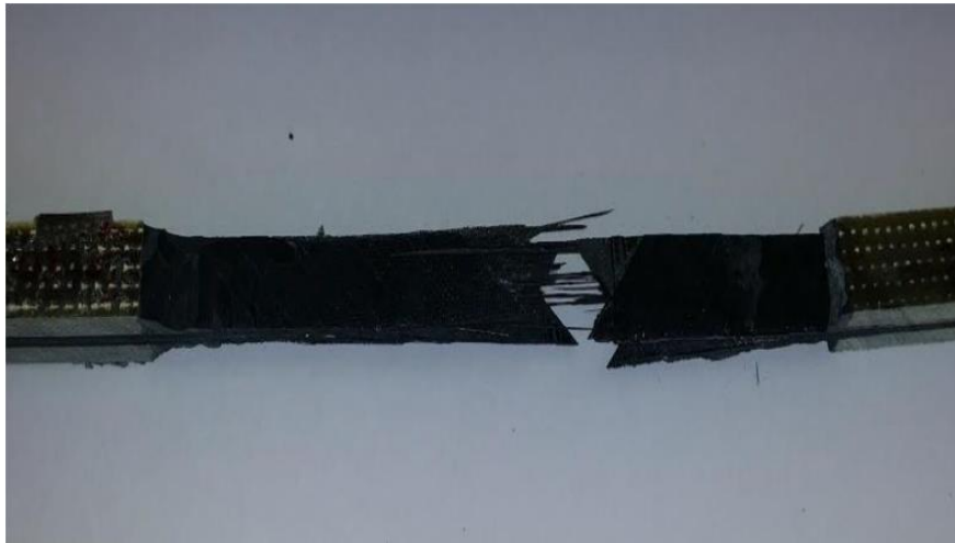
Experimental results of crack and delamination
