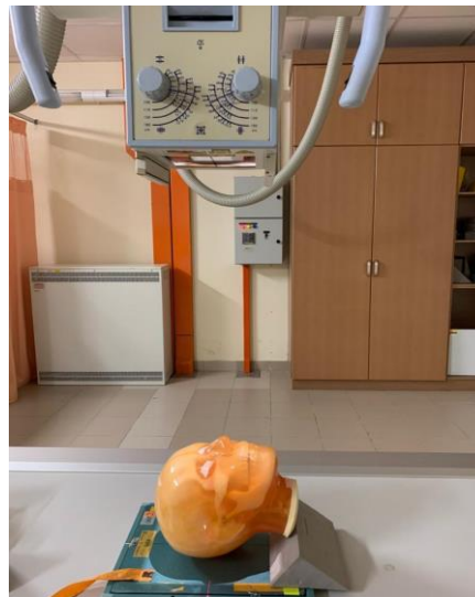
Figure 1. Shows the PBU-50 head phantom on the bucky table with grid (no air gap).
