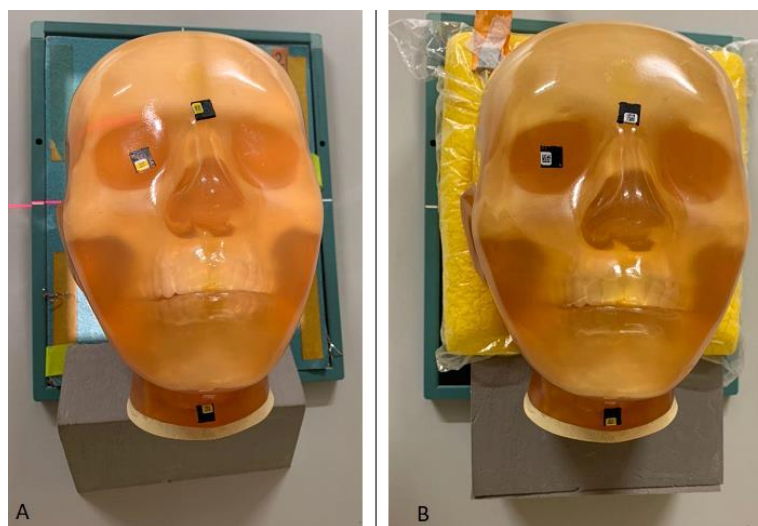
Figure 3. Positions of nanoDot OSLDs on PBU-50 head phantom for the measurement of ESD with a grid (A) and without a grid (B).
