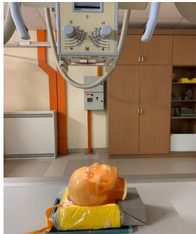
Figure 2. Shows the PBU-50 head phantom on the bucky table without grid with air gap (4cm OID)
