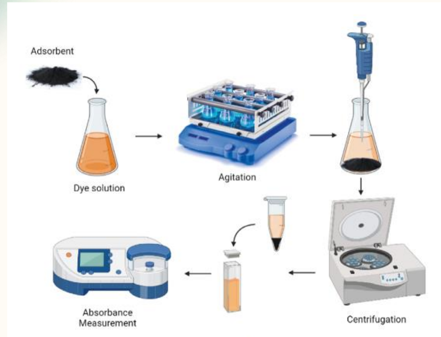
Figure 5: Schematic representation of the adsorption experiment (Khalfaoui et al., 2022)
