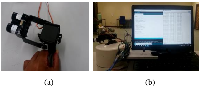
Fig 2. LiDAR sensor calibration with servo motors. Fig 2 (a) LiDAR sensor with 2 servo motors & Fig (b) LiDAR sensors with Arduino for features extraction.
