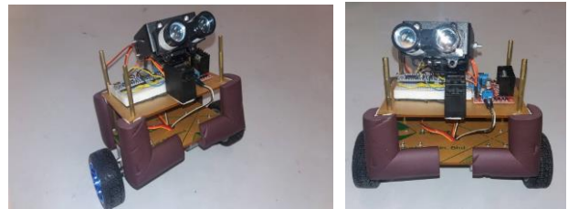
Fig 3. First mobile robot prototype with LiDAR sensor for object recognition.
