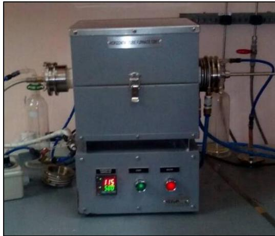
Figure 1: Tube furnace for nitriding process
