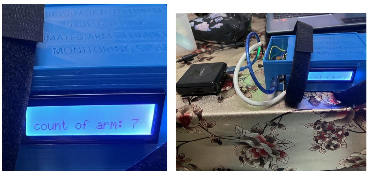
Figure 4.5: Results are displayed on an LCD and a project tool connected to a power bank
