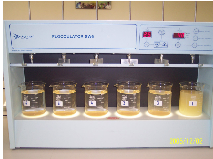
Figure 3. Jar test for high turbidity river water
